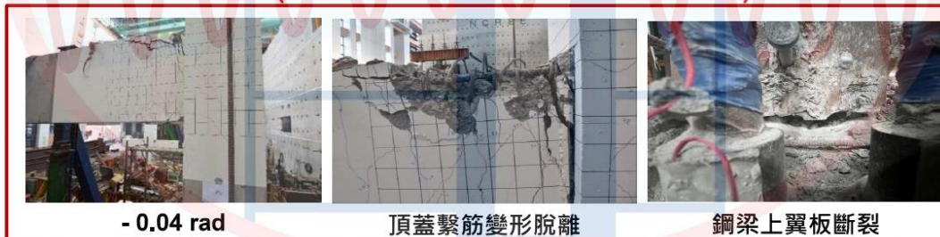
試體1 (No RBS in SRC Beam · 翼板破裂)
