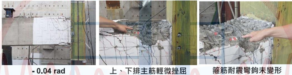
試體1 (No RBS in SRC Beam · 翼板破裂)
